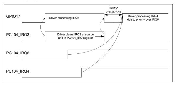
There is a delay of 250-375ns between the de-assertion of the GPIO17 IRQ signal and its new assertion due to the pending PC104 interrupt. This delay is introduced into the ZEUS hardware implementation to accommodate for the minimum inactive time of GPIO signals required by a PXA270 processor (154ns).
